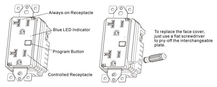
Always-on Receptacle: always connected, not be controlled by button or APP, switch or program button.
